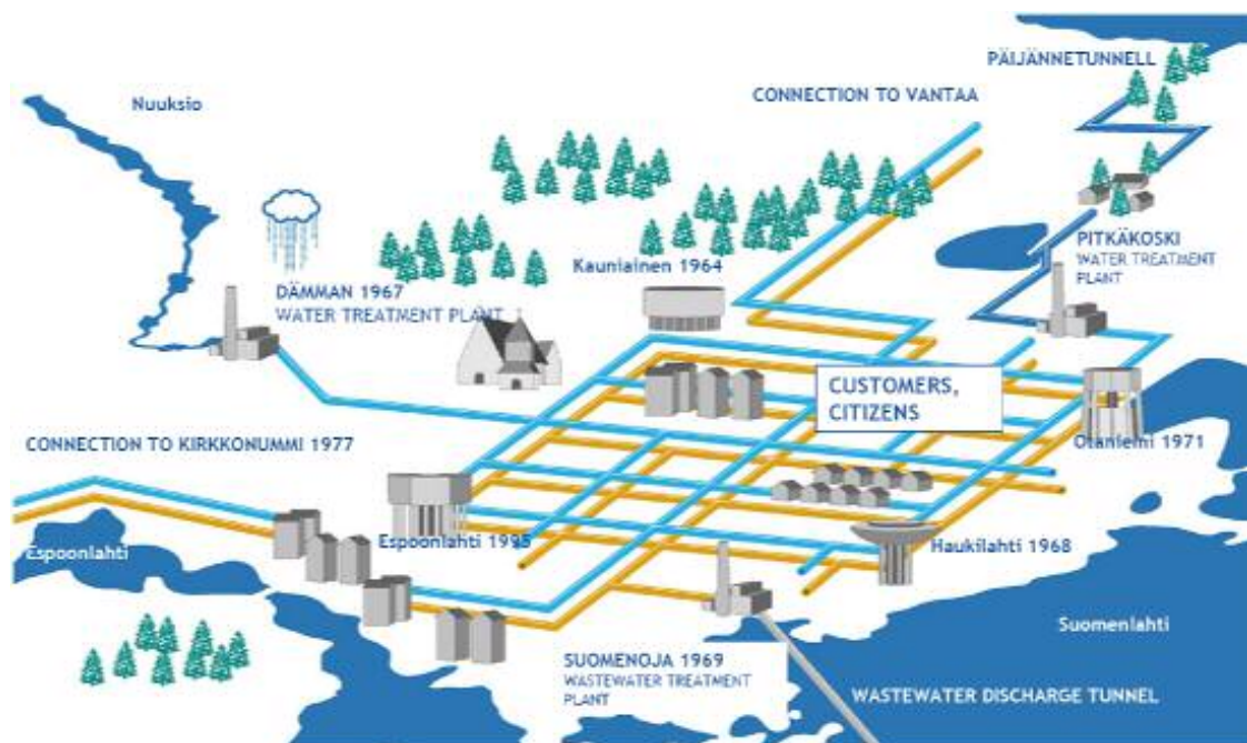
Figure 2. Distribution system of Espoo Water. (Espoo Water 2007)
